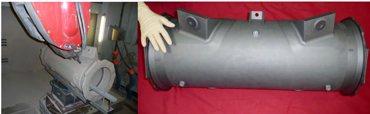
Figure 3. One of the 19 GAIA torus segments (left) during green machining, (right) ready for brazing assembly
