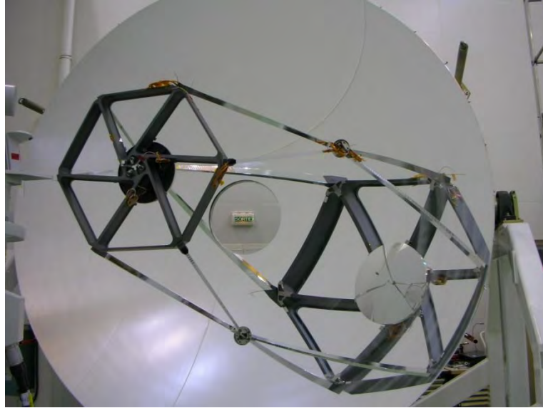
Figure 8. Top view of the hexapod, the bolted M2 and their distorted image in M1
