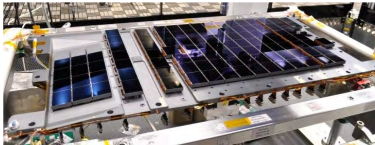
Figure 14. The CCD flight models integrated on the SiC CCD supporting structure
