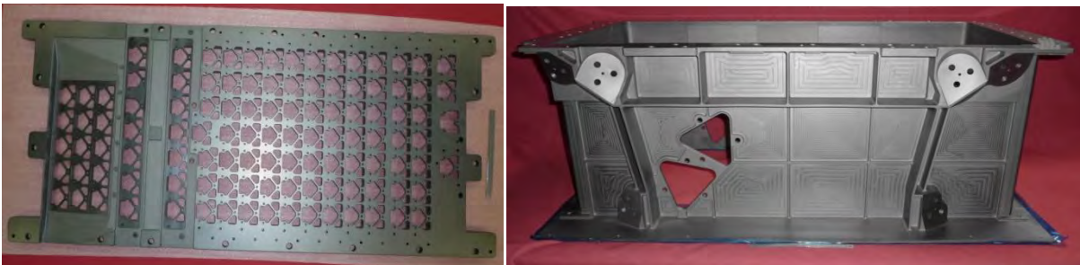
Figure 12. Focal Plane Left ) The CCD supporting structure (1.15 m x 0.53 m - 11 kg) Right ) The Cold Radiator (1.17 m x 0.62 m x 0.41 m - 38 kg)
