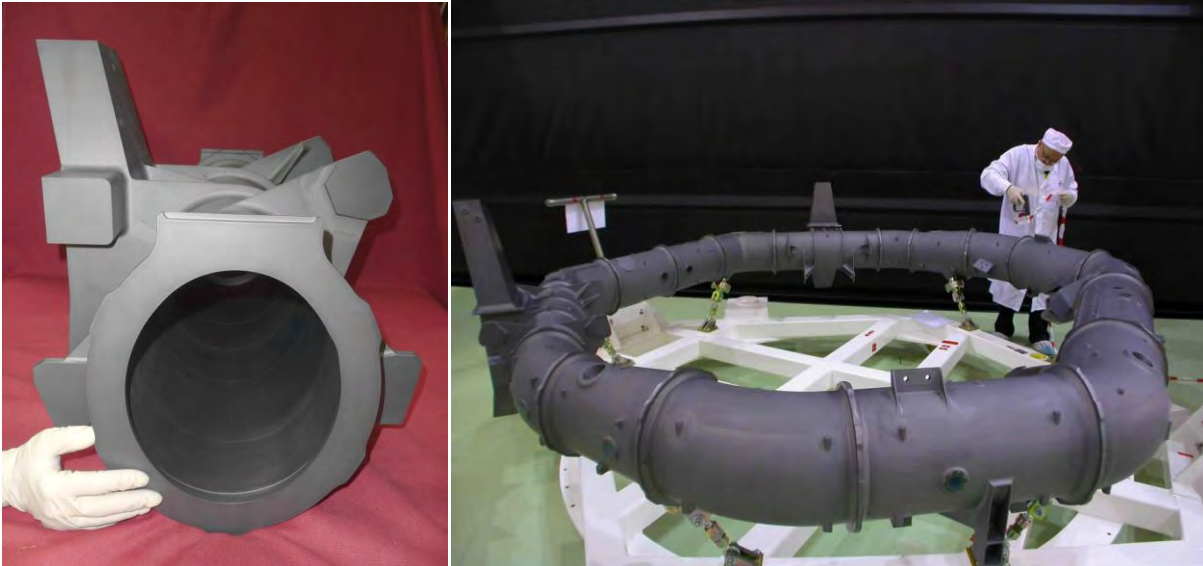
Figure 11. Torus Left ) Torus segment before brazing Right ) Reception of the torus assembly in ASTRIUM (< 200 kg)
