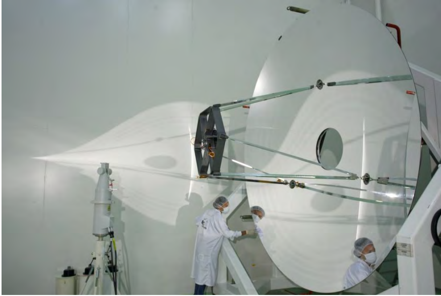
Figure 6. HERSCHEL all-in-SiC telescope
