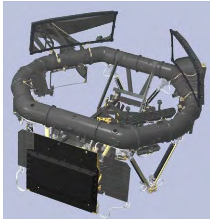
Figure 9. The GAIA payload module features “all SiC” architecture
