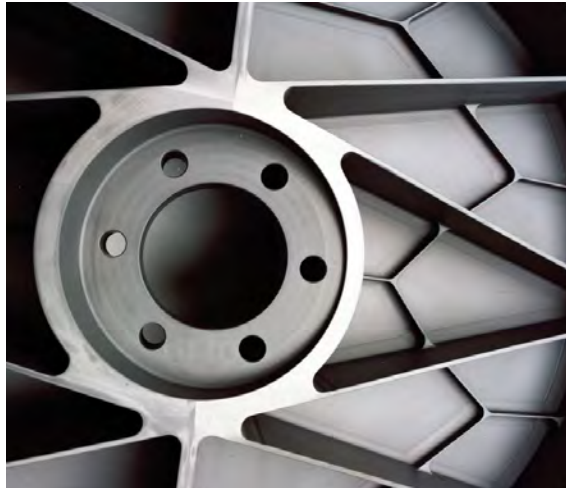
Figure 7. Detailed view of the rear face of HERSCHEL \Phi 3.5 m primary mirror, including an interface
