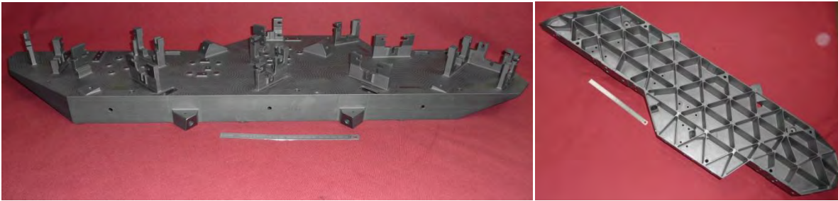
Figure 13. Views of the largest BAM base-plate (0.92 m x 0.28 m - only 5.6 kg)
